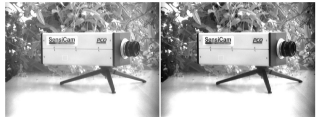
Figure 4 Left image: scaled to full scale 0 - 4095 => 0 - 255 Right image: scaled to minimum - maximum 604 - 4095 => 0 - 255 exposure time = 500 ms (for white rectangle see legend figure1)
