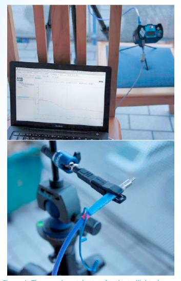
Figure 1. The experimental setup for the twilight observations comprises the Jaz spectrometer, the fiber feed and the data-taking laptop. These photographs, taken around the time of sunset with a "daylight" white balance setting on a Canon 5D Mark II, illustrate the high color temperature of the ambient light at sunset, which is caused predominantly by the ozone absorption (Figure 2).
