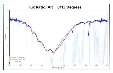
Figure 4. The observed ratio (dark blue), with a normalized continuum, of a spectrum taken with a solar altitude of-3° is compared to one at +13°. Atmospheric models [4] using the HITRAN database (cfa.harvard.edu/hitran) [5], with similar but pure transmission geometry, are over plotted (red: pure ozone absorption; light blue: ozone + O2 + H2O). The models have been scaled in intensity by a factor of 1.7 as a way of accounting for the simplification of the model geometry.
