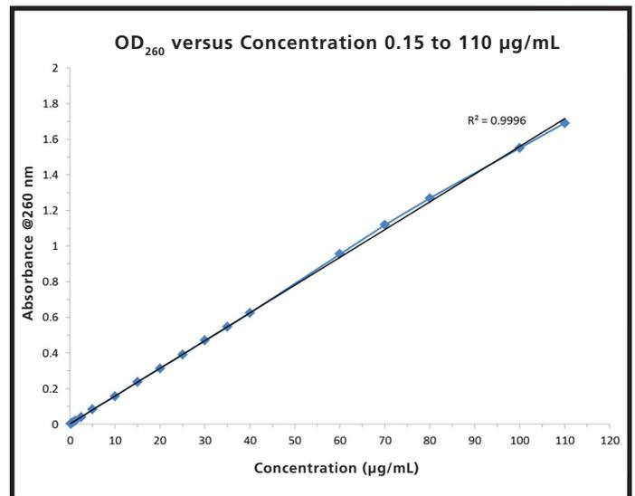
Figure 3: OD<sub>260</sub> versus DNA concentration for concentrations ranging from 0.15 to 110 µg/mL DNA in water
