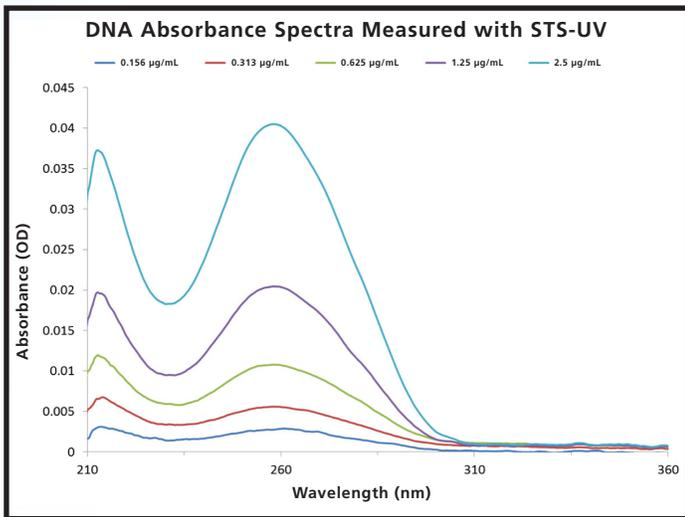
Figure 1: Low concentration (0.15 to 2.5 µg/mL) DNA solution absorbance measured with STS-UV
