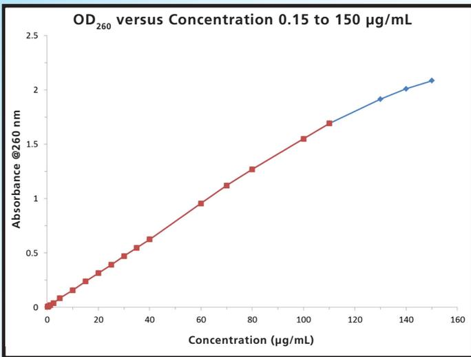
Figure 4: OD<sub>260</sub> versus DNA concentration for concentrations ranging from 0.15 to 150 µg/mL DNA in water
