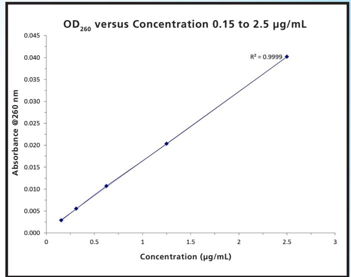
Figure 2: OD<sub>260</sub> versus DNA concentration for concentrations ranging from 0.15 to 2.5 µg/mL DNA in water
