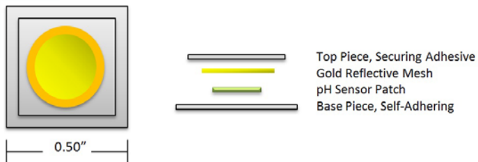
Figure 1: Optical pH sensor includes an electroformed gold mesh applied atop the sensor layer (inset), which both admits the sample and reflects the probe signal.
