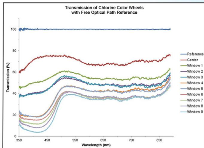
Figure 5: Differences in transmission spectra of chlorine color wheel samples were not as pronounced using air (no wheel) as the reference.
