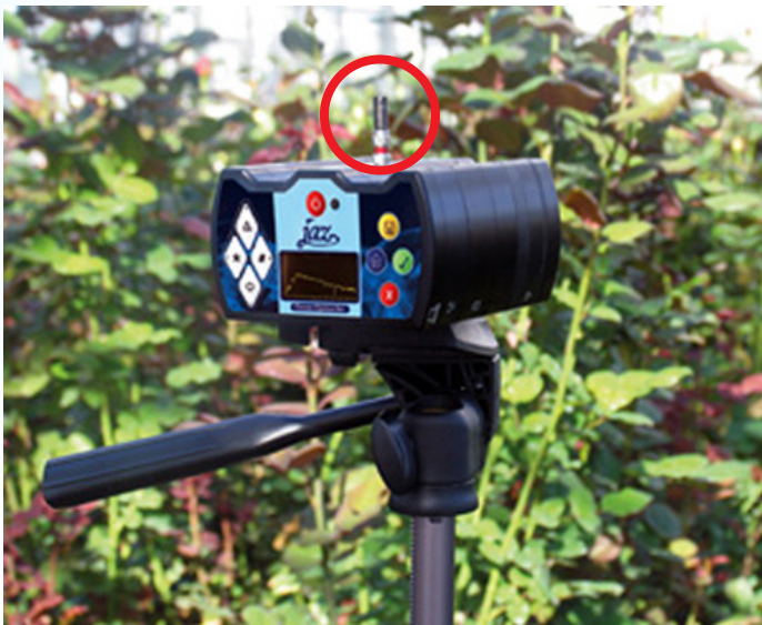
Figure 2: The Jaz spectrometer can be mounted to a tripod and positioned to collect solar radiation from 180° field of view using a cosine corrector attached to the spectrometer.
