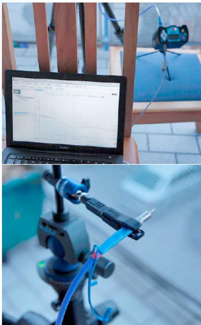
Figure 1. The experimental setup for the twilight observations comprises the Jaz spectrometer, the fiber feed and the data-taking laptop. These photographs, taken around the time of sunset with a “daylight” white balance setting on a Canon 5D Mark II, illustrate the high color temperature of the ambient light at sunset, which is caused predominantly by the ozone absorption (Figure 2).
