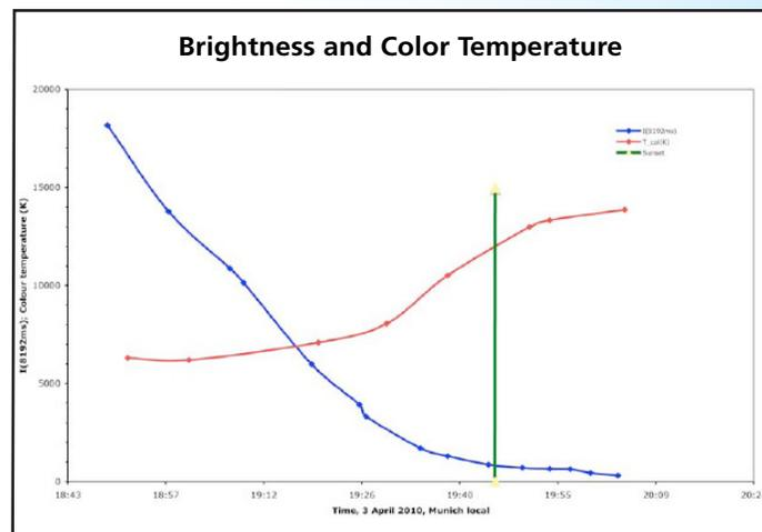
Figure 2. These spectra reveal variation of sky brightness at 700 nm, in units of counts per 8192 ms, and color temperature measured with a Gossen Colormaster 2F color meter.
